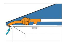
Note: When the summer feature is working the lounge/source room inlet is switched off via the damper and will not receive the cooled air directly from outside, however due to air pressure a natural re-circulation occurs throughout the home.
